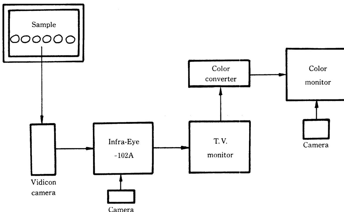
Fig. 1. Block diagram of experimental arrangement of the infrared measurement.
