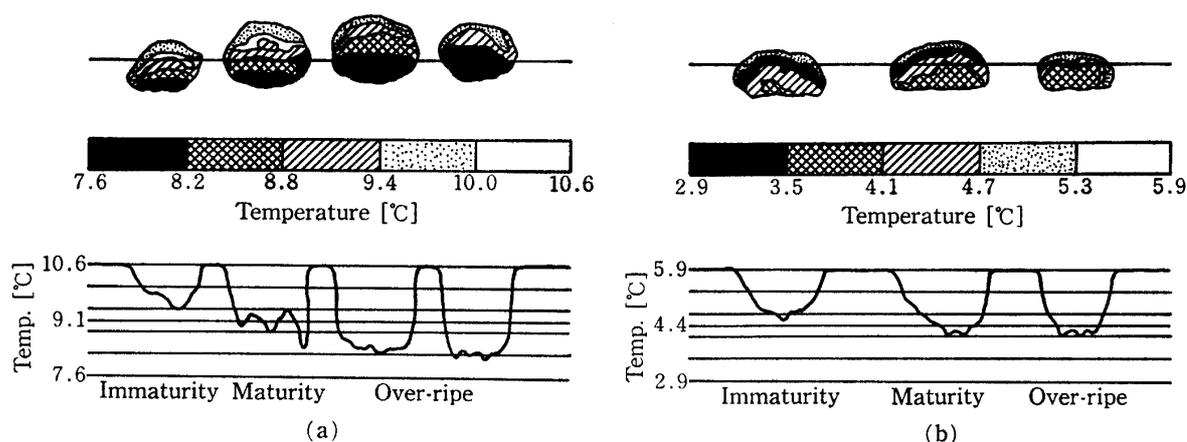
Fig. 7. Thermal images and temperature-curves for Japanese persimmon (cv. Hiratanenashi).
