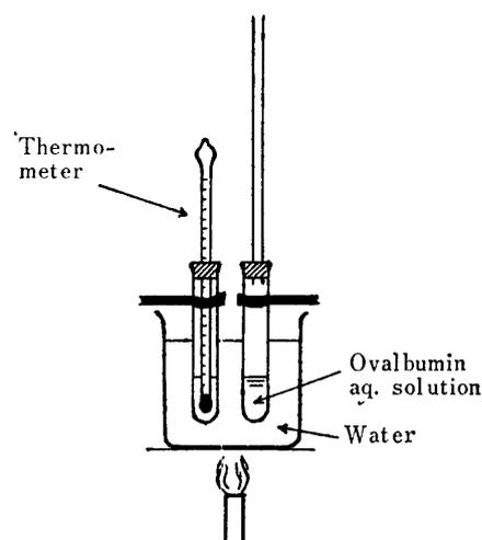
Fig. 1. Equipment for the measurement of the heat-coagulating point of ovalbumin.
