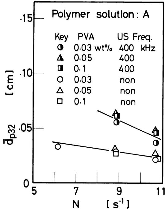
Fig. 4 Effect of PVA concentration on  $\bar{d}_{p32}$  using Solution A as dispersed phase experiment. As might be expected from Eq. (1), the size of droplets is significantly affected by the interfacial tension. From the fact that the interfacial tension of the polymer solution is scarcely affected by the PVA concentrations in the range 0.03~0.1 wt% as shown in Table 3, the above mentioned tendency of average droplet size seems to be not so surprising.
