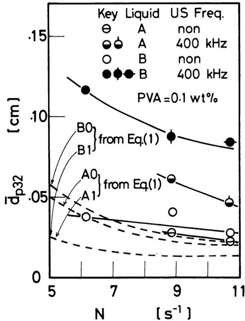
Fig. 2 Effect of ultrasonic irradiation on  $\bar{d}_{p32}$  using polymer solutions as dispersed phase ( A0, A1 : Solution A, and no PVA and 0.1 wt% PVA, respectively, B0, B1:Solution B, and no PVA and 0.1 wt% PVA, respectively )
