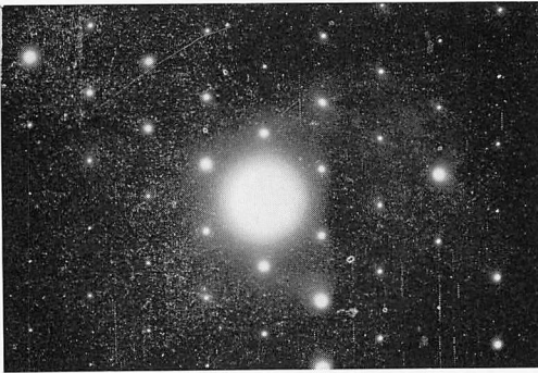
Fig. 9 A representative diffraction pattern observed in 2H-NbSe_2 used for electron microscopic investigations. The spots on the hexagonal grid nearest to the direct beam are 10.0 type and those on the hexagonal grid next to it, are of the 11.0 type.
