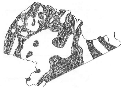
Fig. 7. The distribution of the time averaged water surface elevation at the ninth period calculated by EWM. The shaded (unshaded) area denotes the high (low) water surface region.
