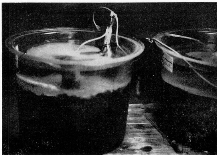
Fig. 1. Experimental equipment for a keeping. The synthetic resinous basin possesses a thermostat, a heater and a bottom filter composed of the upper sand layer, the lower pebble layer and the central air tube. The last contains an air-stone. With a ventilation, water drains into the bottom and gets out of the central tube.
