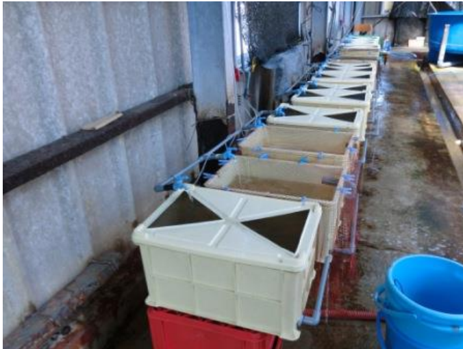
Figure 4.1 Tanks set-up for individual EDC exposure
