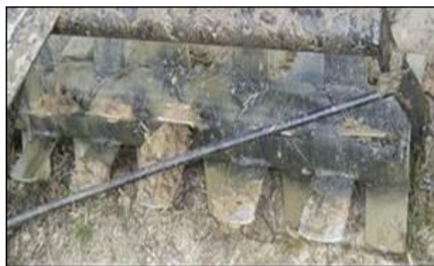
Figure 4.16. Broken puddler during puddling operation
