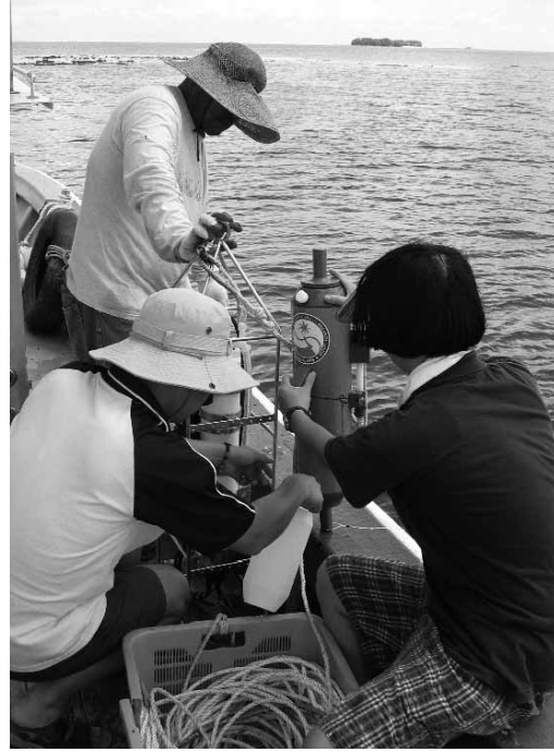
Fig. 6 (left). Local assistants trained in CTD operation. CTD with attached PAR sensor, fluorometer, and beam transmission recorder is manually deployed and retrieved.
