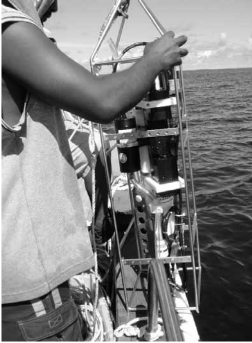
Fig. 6 (left). Local assistants trained in CTD operation. CTD with attached PAR sensor, fluorometer, and beam transmission recorder is manually deployed and retrieved.
