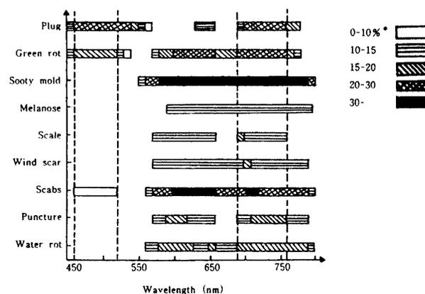
Fig. 3. Selection of wavelength for detection of defects.
