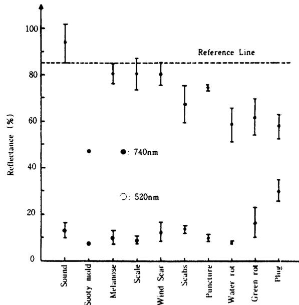
Fig. 8. Reflectance at 740 and 520nm for different defects.
