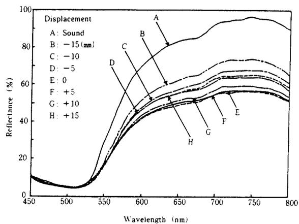
Fig. 7. Spectral reflectance curves for different location of defects on Satsuma mandarin surface. (Left: movement on X-axis, Right: movement on Y-axis)
