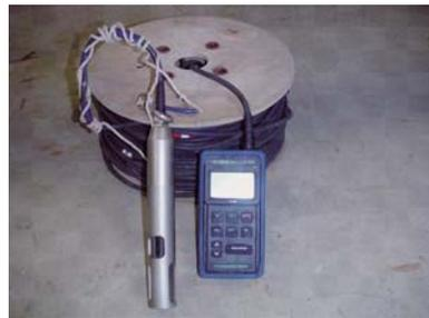
(d). Water temperature and electric conductivity meter
