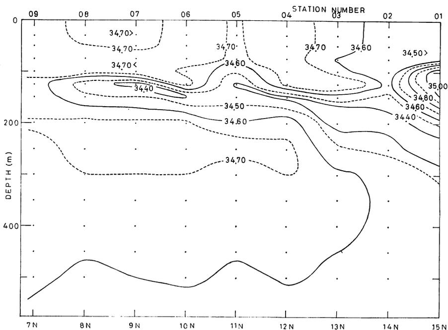
Fig. 3. Salinity distribution (‰) between 7°N and 15°N along the meridian of 158°W.
