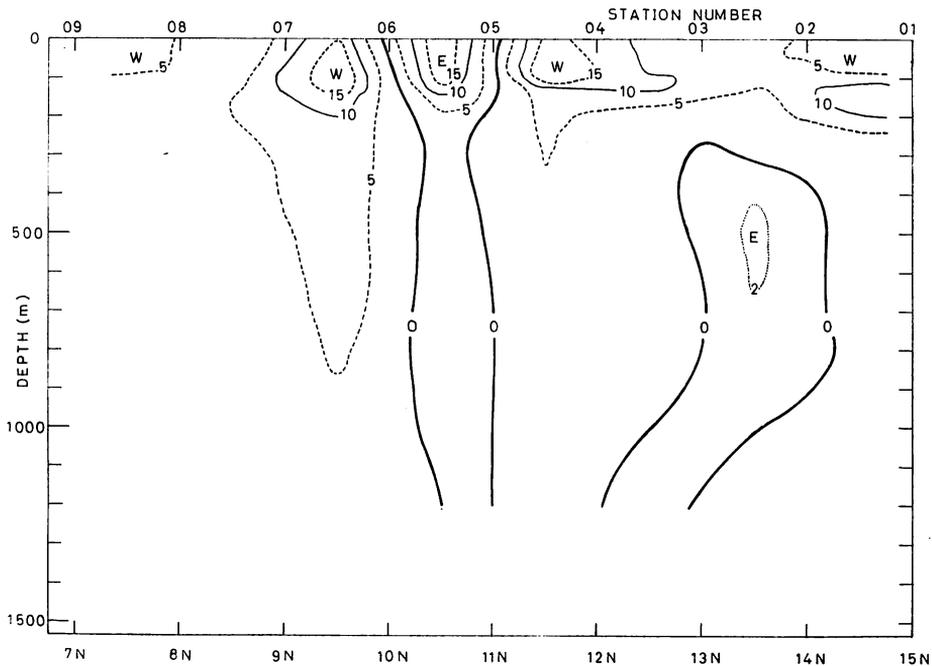
Fig. 5. The east-west component (cm/sec) of calculated relative current velocity across 158°W referred to 1,500m.
