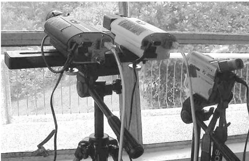
Fig.10. Three cameras at Mayon Volcano Observatory. From the left to the right, near-infrared and visible network cameras connected to the hub, and a video camera standalone. The power is provided through uninterrupted power supply.
