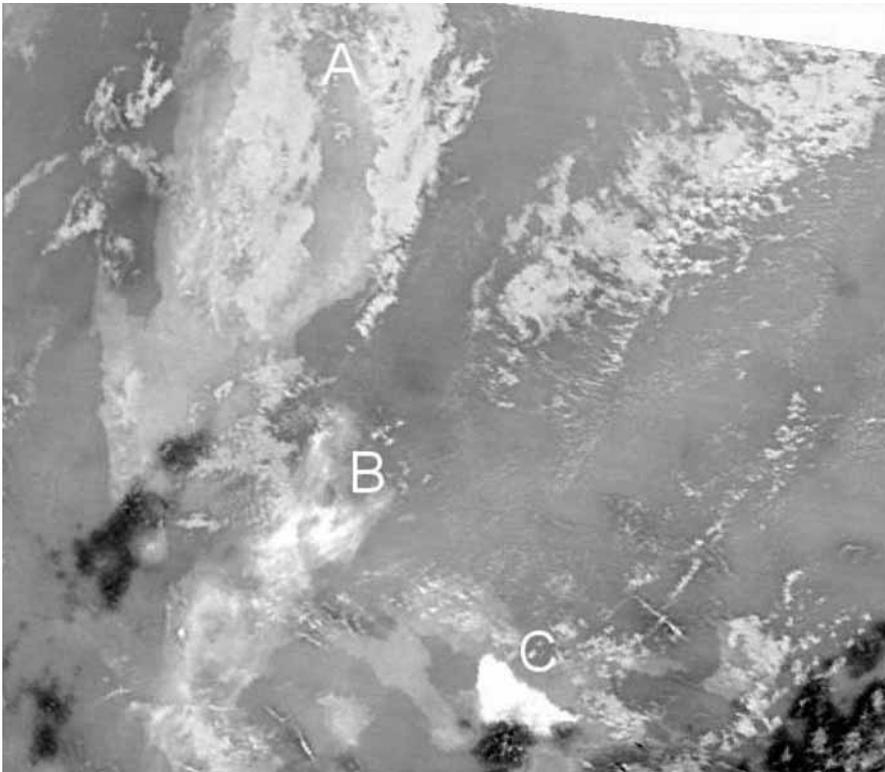
Fig.4. Contrast-stretched 1730 UTC NOAA-14/AVHRR image of 12-11  $\mu\text{m}$  brightness temperature differences, corresponding to the last image in Fig. 1. Negative differences are shown in white. Data courtesy NOAA.
