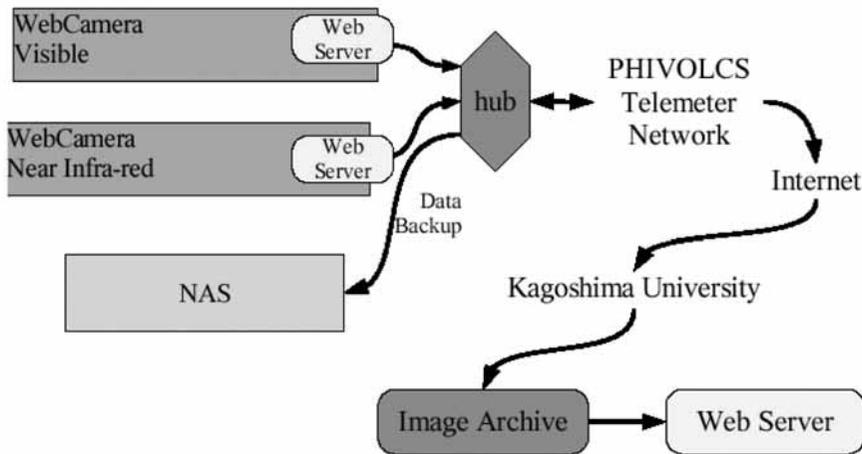
Fig.11. Network camera system connected with Internet.
