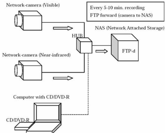
Fig.8. System design for visible and near-infrared network camera system.
