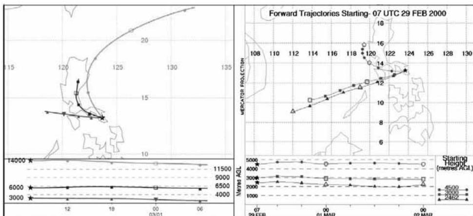
Fig.3. Forecast trajectories for clouds from the 0701 UTC eruption. Left panel: NOAA/HYSPLIT display using FNL data, trajectories starting at 3000, 6000, and 14000 metres. Right panel: Bureau of Meteorology HYSPLIT using LAPS data, trajectories starting at 2462 (mountain top), 3000, and 4500 metres.
