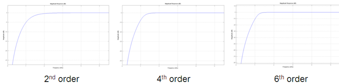
Fig. 15 Butterworth filters of 2 nd , 4 th and 6 th order. We can notice that a 2 nd order filter is too smooth while the 6 th order compromises the information in the signal
