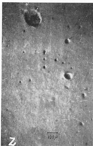
Fig. 10. Example of the sampling surface of the MgO film with the craters developed by sea-salt particles. The scale indicates 100\mu .
