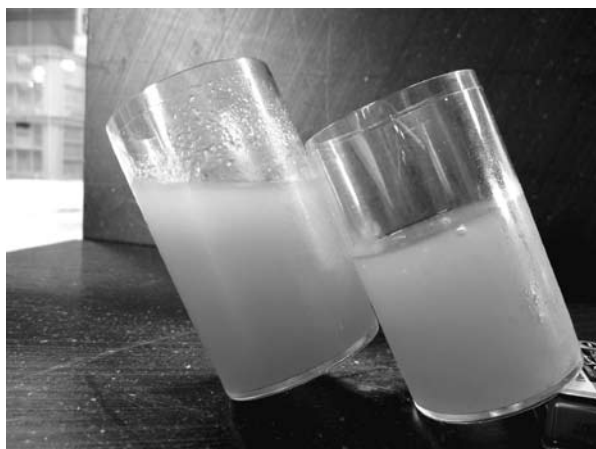
Fig. 3. Water containing non-treated papaya fruit powder was solidified with agar (right) but not solidified with gelatin (left).
