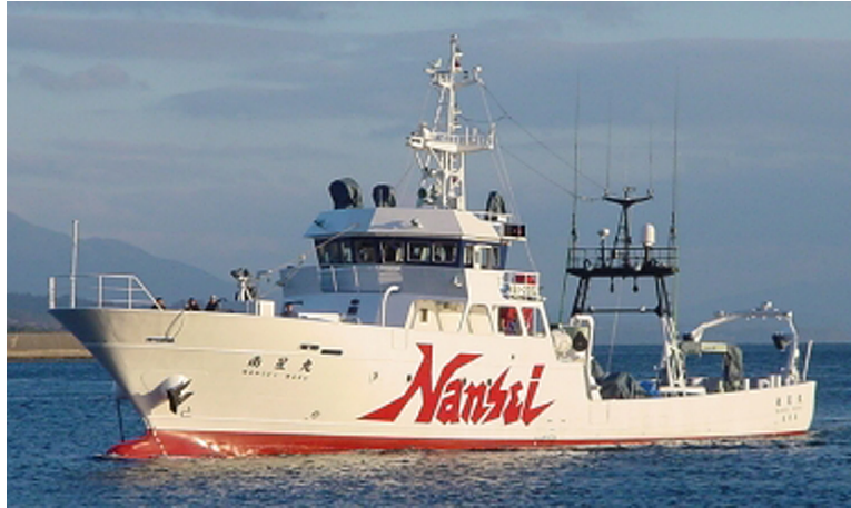
Plate 1. The training ship Nansei Maru. (175GT, Length/ 41.96M, Breadth/ 7.50M, Depth/3.3M, Capacity/ 30 persons)
