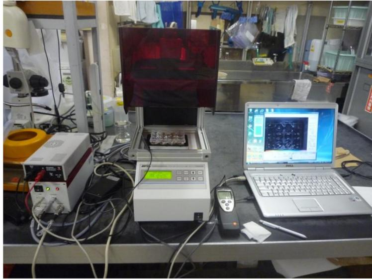
Fig. 3.3. Imaging-PAM used in this study.
