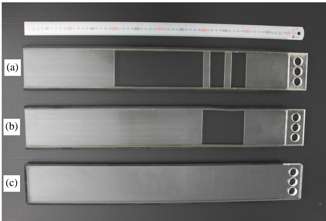
Figure 3.7 Experimental subsurface barriers: (a) 20 cm cutoff wall, (b) 40 cm cutoff wall and (c) shutoff wall.
