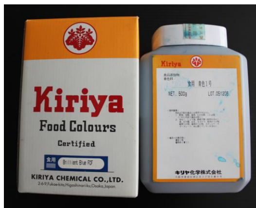
Figure 4.3 Blue food color used to dye the freshwater recharge.
