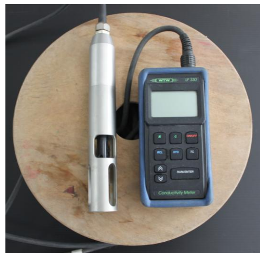
Figure 3.5 WTW-LF330 conductivity meter.
