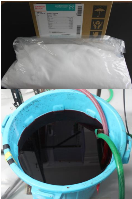
Figure 3.2 Saltwater in 40 L barrels made from commercial salt dissolved in tap water.
