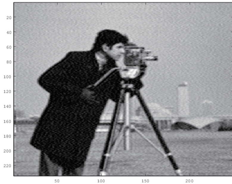
Fig.7 Restored image by the RLS Wiener fixed-point smoother for SNR=20 [dB] and Lag=3.
