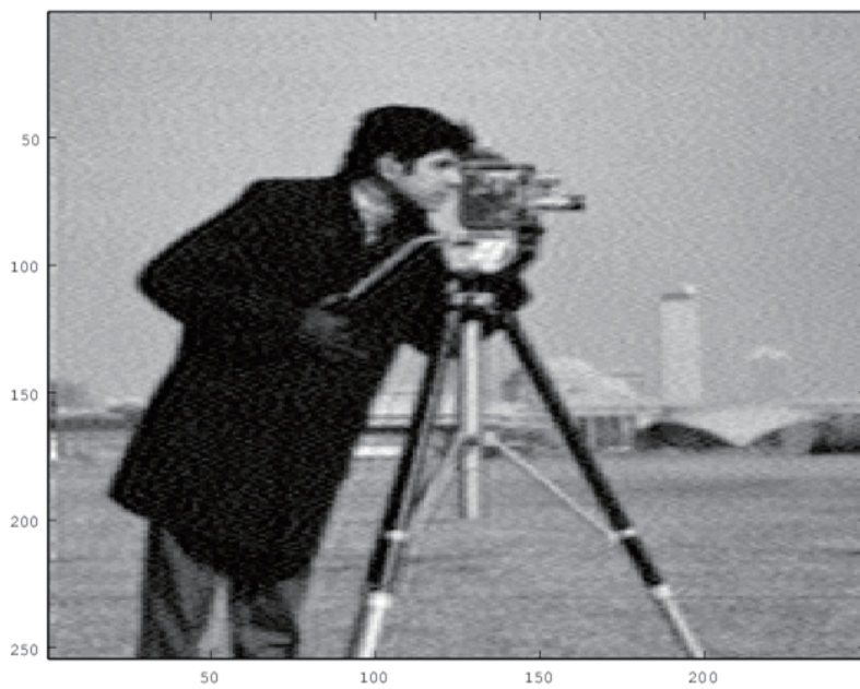
Fig.10 Restored image by the RLS Wiener fixed-point smoother for SNR=30 [dB] and Lag=3.
