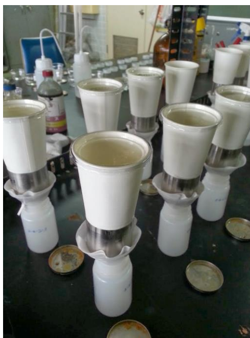
Figure 31: Soil solution extraction from undisturbed soil column
