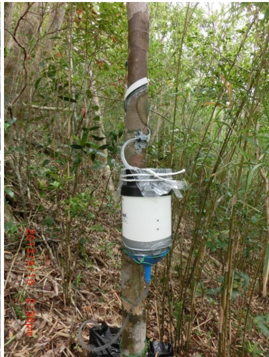
(d) Stemflow gauge attached to a collector
