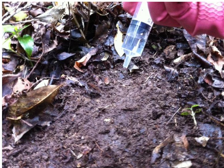
Figure 12: Field measurement of soil water repellency by water drop penetration time test
