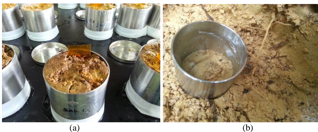
Figure 32: In vitro (a) and in situ (b) application of ion exchange membrane technique
