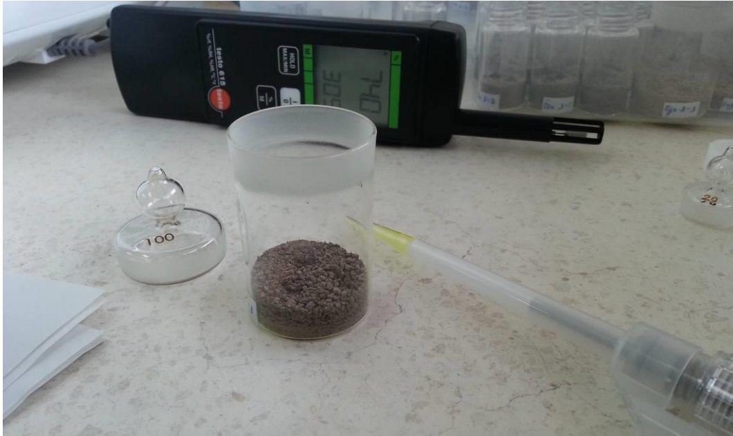
Figure 13: Laboratory water drop penetration time test
