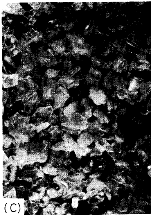
Photo 1. Microphotographs of samples, (A) Toyoura sand, (B) Nejime beach sand, (C) Shirasu-A, and (D) Shirasu-B.
