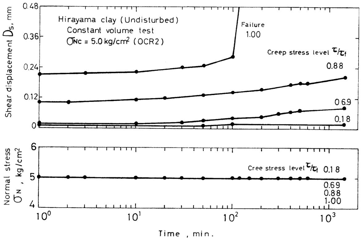
Fig. 6. Shear displacement, normal stress versus logarithmic time in the residual state of undisturbed Hirayama clay.
