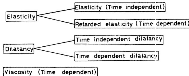
Fig. 7. Components of creep deformation.
