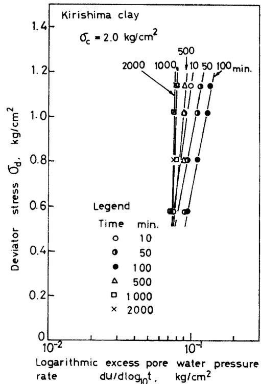
Fig. 9. Relationship between deviator stress and logarithmic excess pore water pressure rate for normally consolidated Kirishima clay.
