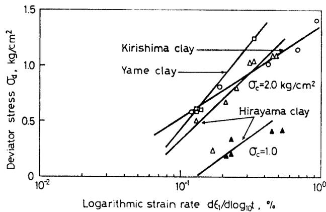
Fig. 11. Relationship between deviator stress and logarithmic strain rate for normally consolidated clays.
