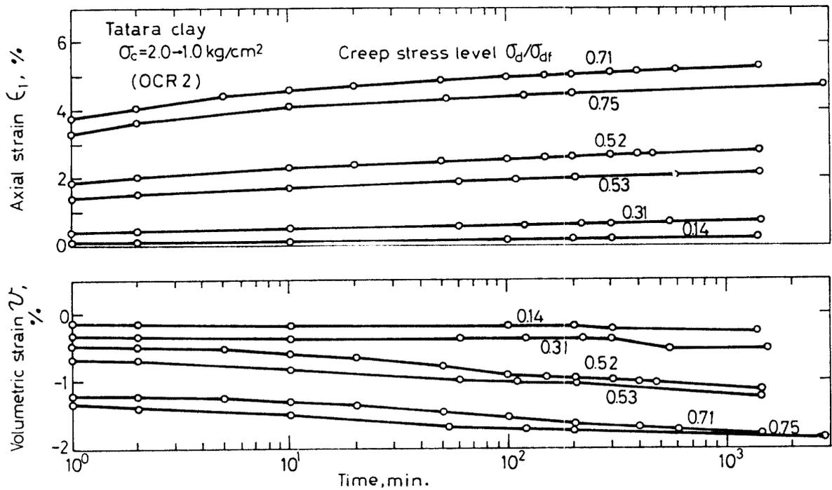
Fig. 4. Axial strain, volumetric strain versus logarithmic time for over-consolidated Tataro clay.
