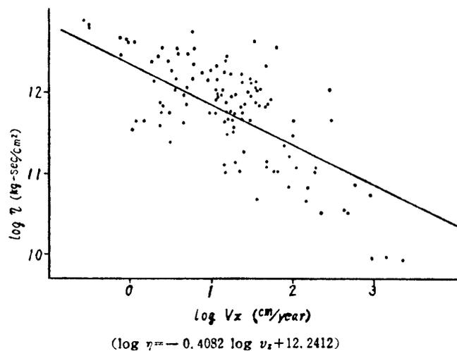
Fig. 27. Relationship between viscosity  $\eta$  and an annual displacement  $V_z$  of landslides (after Takenouchi<sup>35)</sup>).
