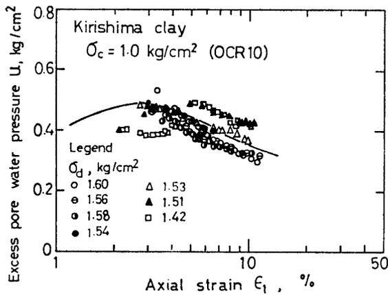
Fig. 18. Relationship between excess pore water pressure and axial strain for over-consolidated Kirishima clay.
