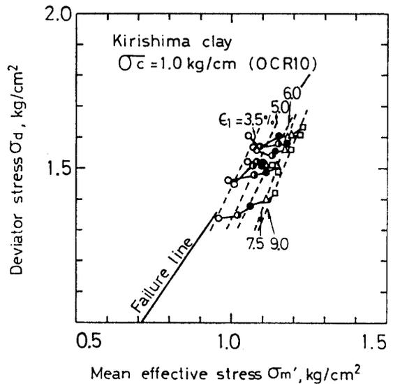
Fig. 19. Stress paths of creep failure for over-consolidated Kirishima clay.
