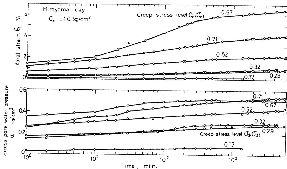
Fig. 2. Axial strain, excess pore water pressure versus logarithmic time for normally consolidated Hirayama clay.
