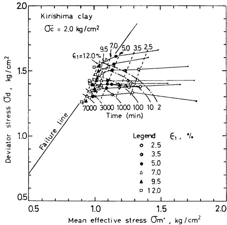
Fig. 14. Stress paths of creep failure for normally consolidated Kirishima clay.
