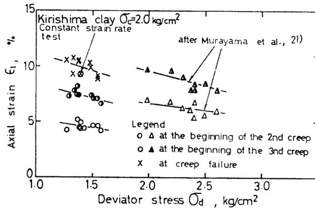
Fig. 21. Influence of deviator stress on axial strains at the beginning of the second and third creep and creep failure for normally consolidated clays.
