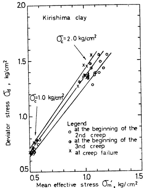
Fig. 20. Effective stresses at the beginning of the second and third creep and creep failure for normally consolidated Kirishima clay.
