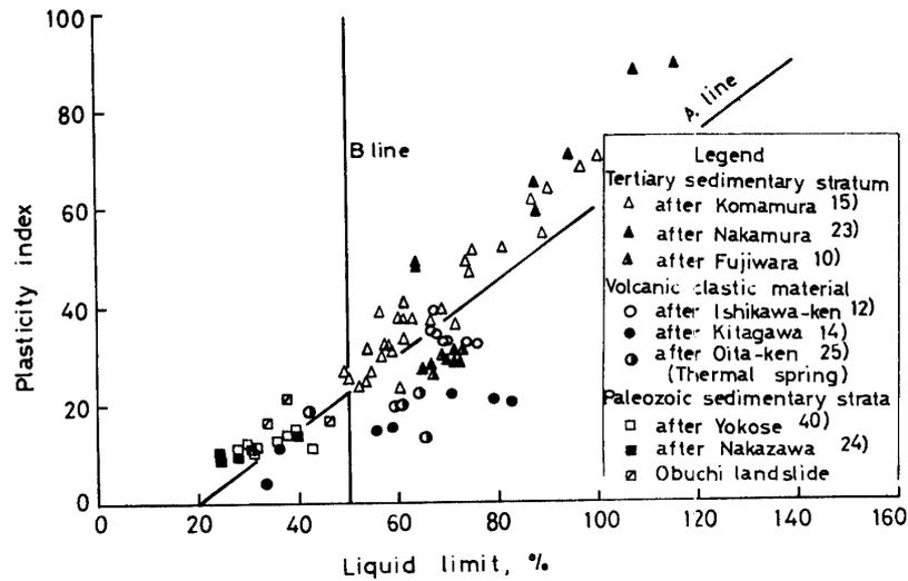
Fig. 28. Plasticity chart of landslide clays.
