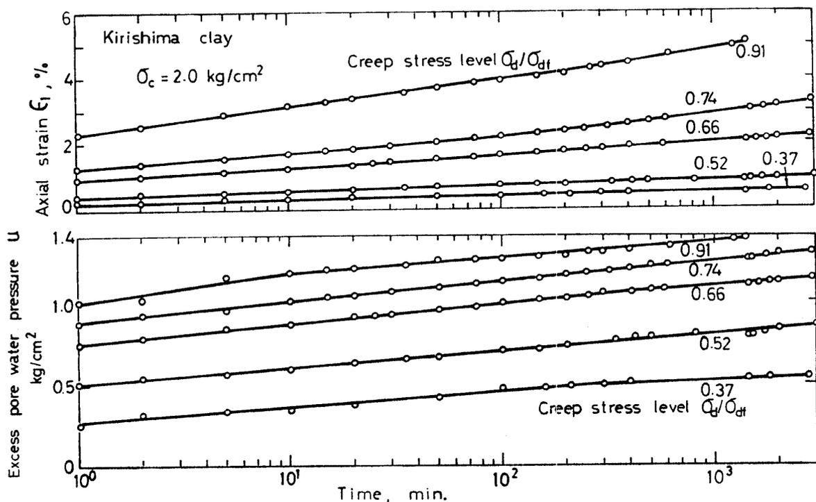
Fig. 1. Axial strain, excess pore water pressure versus logarithmic time for normally consolidated Kirishima clay.
