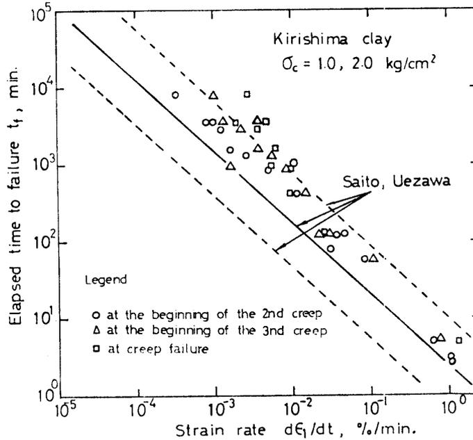
Fig. 26. Relationship between axial strain rate and elapsed time to creep failure for normally consolidated Kirishima clay.
