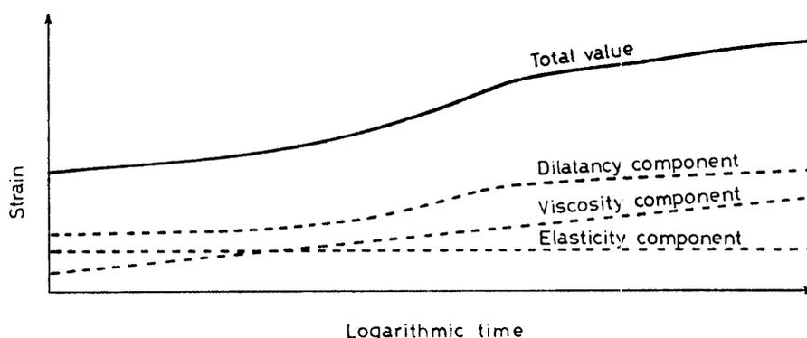
Fig. 10. Schematic representation relating the components of creep deformation versus logarithmic time.
