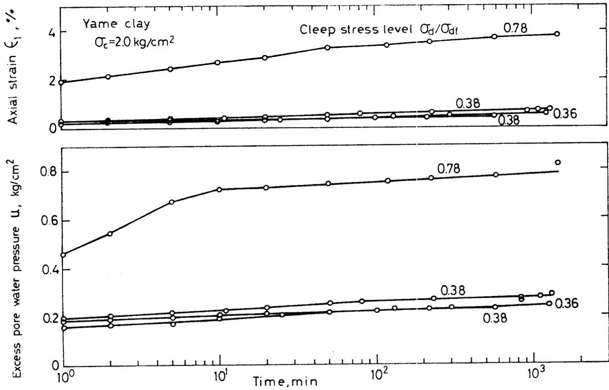
Fig. 3. Axial strain, excess pore water pressure versus logarithmic time for normally consolidated Yame clay.
