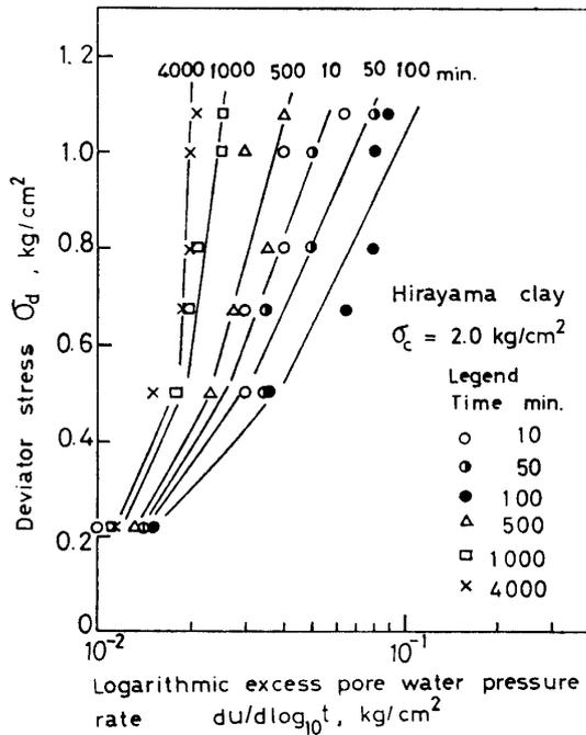
Fig. 8. Relationship between deviator stress and logarithmic excess pore water pressure rate for normally consolidated Hirayama clay.
