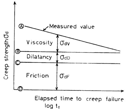
Fig. 22. Schematic representation relating time dependency of creep strength components.
