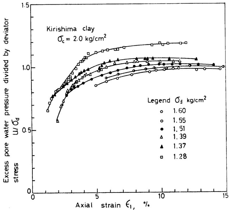
Fig. 16. Relationship between excess pore water pressure divided by deviator stress and axial strain for normally consolidated Kirishima clay.
