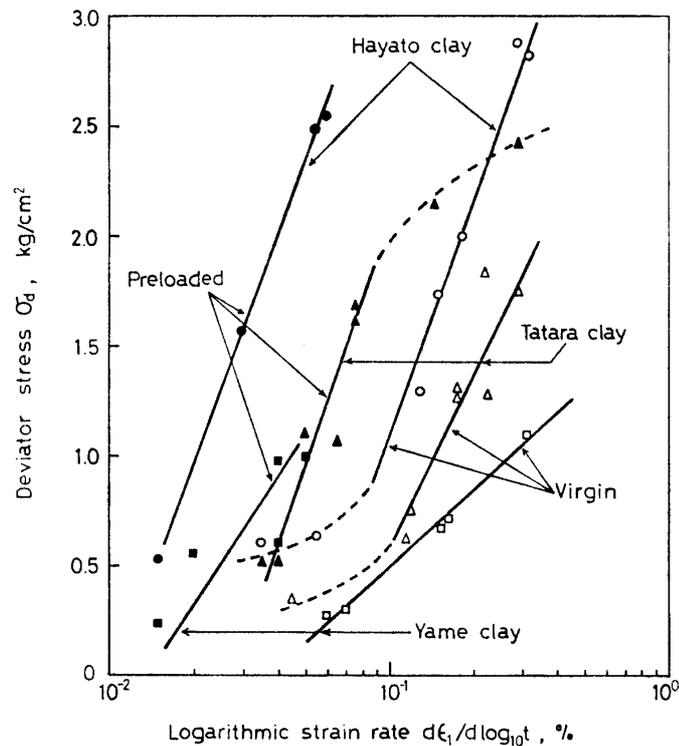
Fig. 12. Relationship between deviator stress and logarithmic strain rate for over-consolidated clays.
