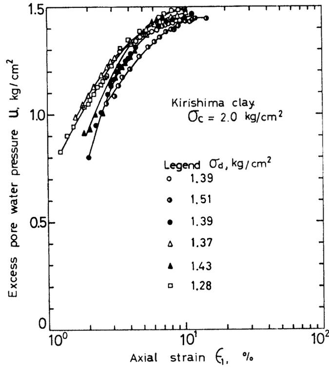
Fig. 15. Relationship between excess pore water pressure and axial strain for normally consolidated Kirishima clay.
