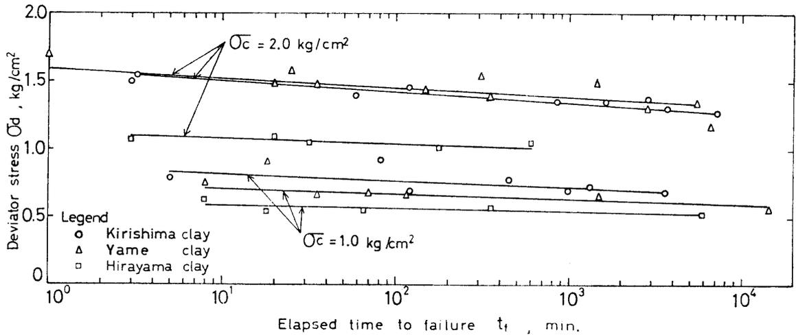
Fig. 17. Influence of elapsed time to creep failure on creep strength of normally consolidated clays.
