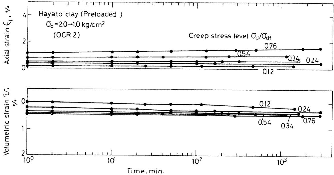
Fig. 5. Axial strain, volumetric strain versus logarithmic time in the preloaded state of Hayato clay.
